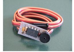
1. With both the transmitter and receiver powered off, plug the servo plug into the receiver channel # to which you want to use as your shutter control. This can either be a switch or joystick controlled channel.
