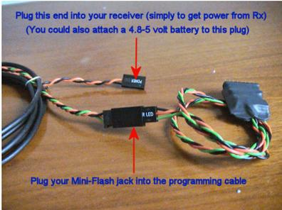
**Step 3:** Connect the POWER end of the programming cable (female plug) to your receiver and be sure the receiver is powered up (this connection to the Receiver simply provides power to the Mini-Flash during the downloading process; you could always use a 4.8v-5v battery instead of connecting it to your receiver)
