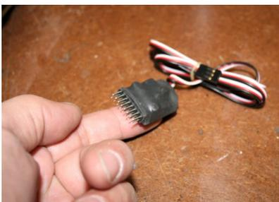
Weighing merely 9 grams and roughly 1 square inch by 1/4" thick, the Mini-Flash is based around a tiny 8-pin programmable microcontroller chip. The controller can get its power from either a R/C receiver or an external battery (normally, it is plugged into a receiver). The Mini-Flash is designed to operate off of a 4.8-5 volt power source therefore do not attempt to run it off of anything else or you will ruin the microcontroller. The Mini-Flash provides for 4
