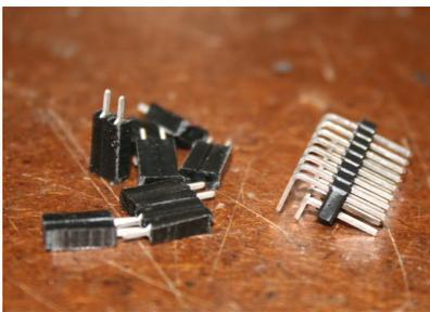
The LED mating connectors supplied provide a nice tight connection to the LED connector pins located on the Mini-Flash. If you are going to heat shrink these ends, be sure you do not cover the black portion of the connector as this will not allow you to plug these connectors side-by-side onto the Mini-Flash (as the heat shrink makes the connectors too wide). If you are only using 4 LEDs (one per channel), you can skip every other row on the Mini-
