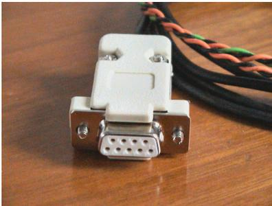
**Step 2:** Connect the programming cable's 9-pin connector (rs-232 serial cable) to an empty RS-232 serial communications port on your computer. Make note of the actual com port number (usually 1 or 2, some PCs could have more), as you will need to define this port in the programming software later if you already haven't changed it.
