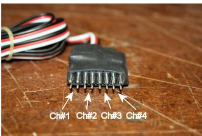
The picture to the left indicates the LED channel outputs. Notice that each of the 4 channels have two outputs, allowing you to connect two LEDs per channel. If you want to add more LEDs to a channel, you will need to either make an adapter (a "Y" adapter or splitter) or simply solder multiple LED lead wires onto the connector. As shown in the picture, the pins along the top are ground (-) while the
